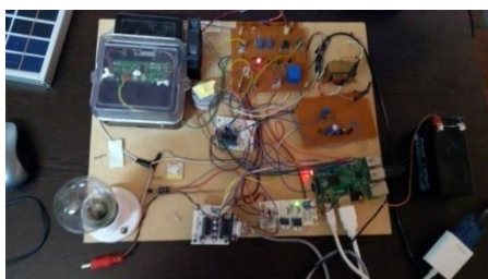
Fig.3. Turn OFF the appliance when current bill exceeds the limits
